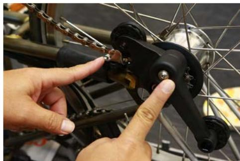
**Step 15.** Place the chain tensioner arm into position to tension the chain as shown.
