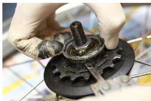
**Step 4.** Remove the large sprocket. Again, take note of the sprocket face orientation to facilitate assembling later.
