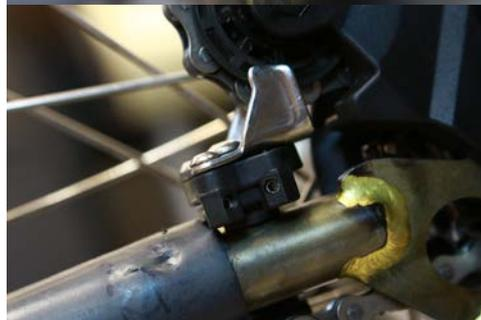
**Step 5.** At the rear derailleur, screw in the high limit screw sufficiently such that the derailleur guide just touches the jockey wheel as shown. The high limit screw is the left screw in the picture shown on the right (bottom).
