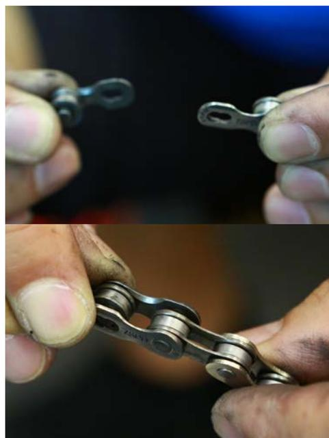
**Step 5.** To complete the joint, gently tension the chain so that the links are closed and locked into position.
