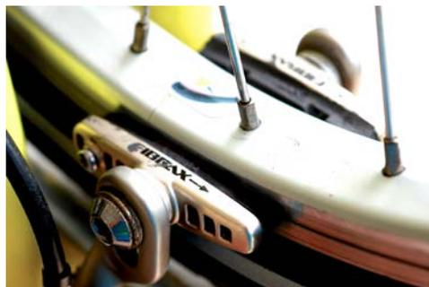
**Step 5.** If the contact is not even, small adjustments to the 'swing' of the brake shoes can be made with a size 2.5mm allen key with this screw.
