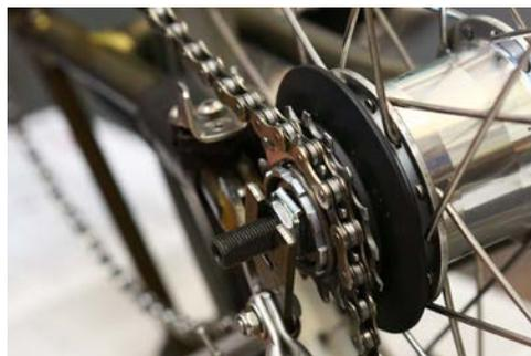
**Step 14.** Install the chain tensioner. Note the position of the chain with reference to the jockey wheels.
