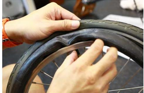
**Step 12.** Insert the rest of the inner tube around the rim and in the tire.
