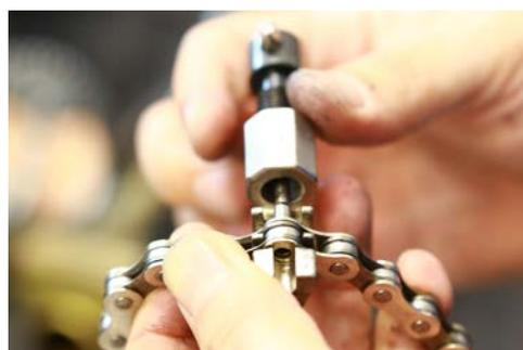
**Step 8.** Holding the chain and chain tool firmly, turn in the handle on the chain tool to push the chain pin into the chain gradually. Stop when the chain pin is almost fully in.
