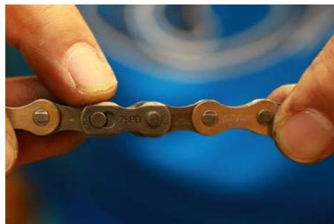
**Step 6.** To separate the chain, hold firmly on the Powerlink surface to slide and unlock the links.
