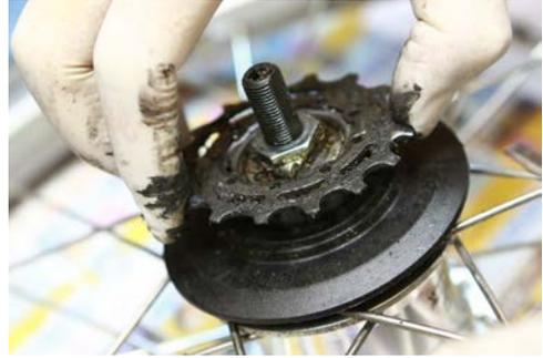
**Step 5.** Finally, remove the plastic guard. The removal process is now completed.
