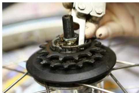
**Step 2.** Remove the small sprocket from the hub. Take note of the sprocket face orientation to facilitate assembling later.
