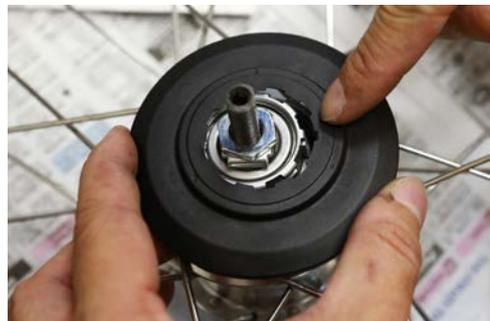
**Step 8.** Similarly, install the large sprocket with the correct orientation as shown. Notice the curvature of the sprocket teeth.
