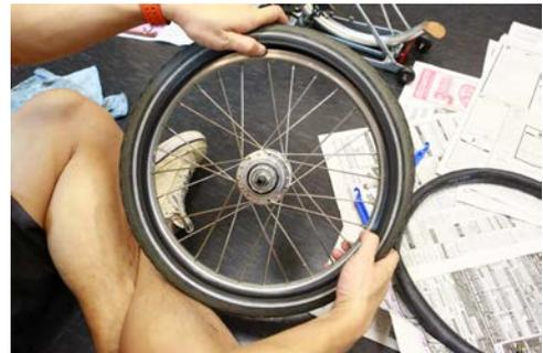
**Step 10.** For rims fitted with the original blue plastic rim tape, use a flat head screwdriver to lift up the rim tape at the valve stem hole to facilitate the ease of inserting the stem valve. You can also apply some grease on the stem valve to do this.
