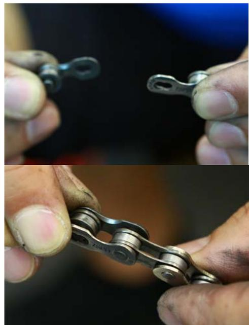
**Step 5.** To complete the joint, gently tension the chain so that the links are closed and locked into position.
