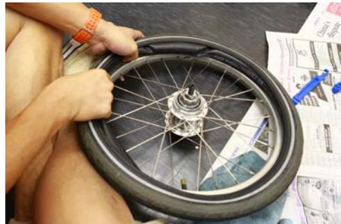
**Step 13.** Start fitting in the bead wall into the rim, beginning from the stem valve end of the tire.
