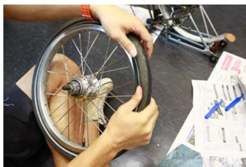
**Step 18.** Do a final visual check that the tire is properly fitted. Install the wheel back to the frame before inflating to the required tire pressure. This is to ensure that the wheel can fit in-between the brake pads.
