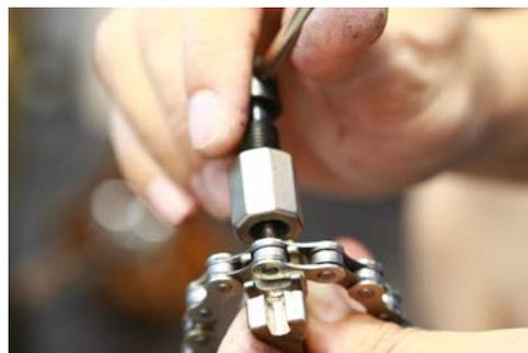
**Step 10.** Making sure that the push pin and chain pin are aligned, turn the chain tool
