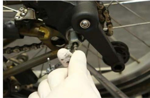
**Step 6.** Remove the chain tensioner with the size 15mm spanner. Set aside the retaining nut and washer.
