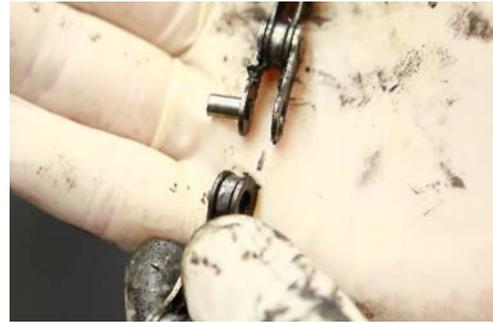
**Step 6.** To join the chain, place the chain in the lower chamber of the chain tool as shown.
