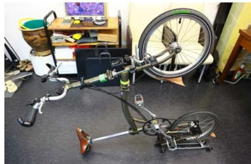
**Step 2.** If you cannot remember the amount of tension on the gear cable barrel assembly with the gear chain rod, adjust the tension by tightening the gear cable barrel to about half the length of gear chain rod screw thread. Do not tighten the lock nut at this time.
