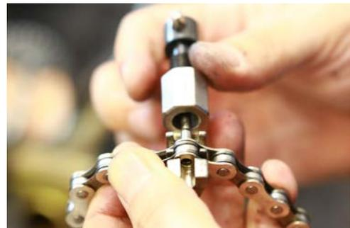
**Step 8.** Holding the chain and chain tool firmly, turn in the handle on the chain tool to push the chain pin into the chain gradually. Stop when the chain pin is almost fully in.
