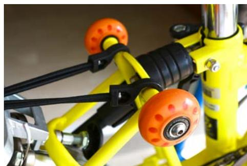
2 important points to note when performing this modification. First is to ensure the diameter of wheel is not excessive (max 72mm is ideal). Otherwise, the bicycle may roll on uneven ground as the rubber stopper at the end of the seat post cannot come into contact with the ground when in fully folded position. Second is the need to have longer
