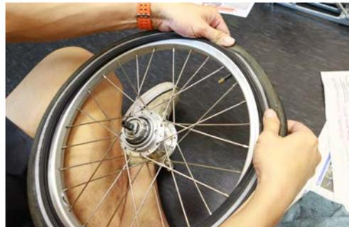
**Step 14.** Use both palms to press in the tire bead wall simultaneously on each side of the rim, working around the rim.
