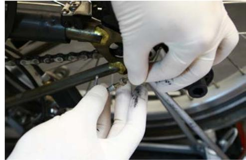
**Step 5.** Unscrew the gear chain rod from the rear hub and set aside for cleaning later.
