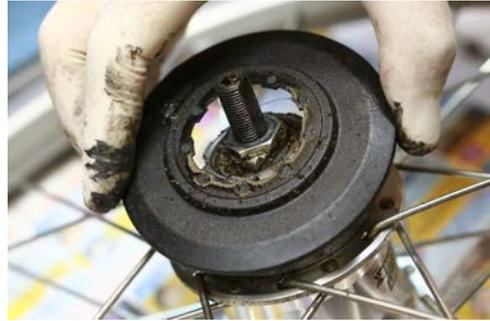
**Step 6.** Clean the hub, sprockets, spacer and spring clip with appropriate degreaser or cleaning agent. Put in your chain too if it needs deep cleaning. Use an old toothbrush dipped in a degreaser to remove stubborn and hard to reach areas is highly recommended.
