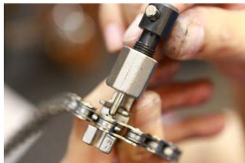
**Step 9.** Remove the chain from the lower chamber. You will notice that the chain link is very stiff and cannot be articulated. That is normal. Move the chain and the affected pin into the upper chamber as shown.
