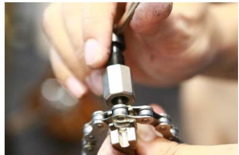
**Step 10.** Making sure that the push pin and chain pin are aligned, turn the chain tool
