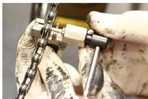
**Step 4.** Remove the chain from the chain tool to check if it can be separated after several turns of the handle. Re-insert the chain into the chain tool and continue pushing the chain pin if necessary. With enough practice and experience, you will be able to do this within a few tries.
