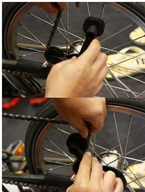
**Step 16.** Next, install the gear chain rod. After screwing in the gear chain rod, turn back a quarter to half turn before connecting the chain with the gear cable barrel assembly. Lock the barrel in position with the lock nut. Installation is now complete.
