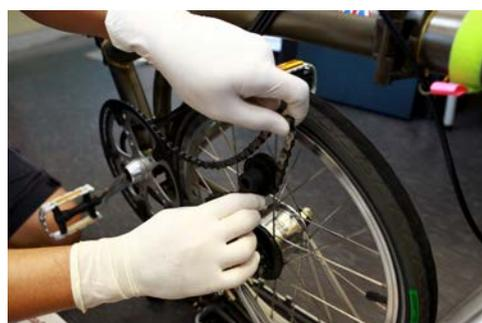
**Step 4.** Unscrew the gear cable barrel from the gear chain rod to disconnect the gear cable from the hub.
