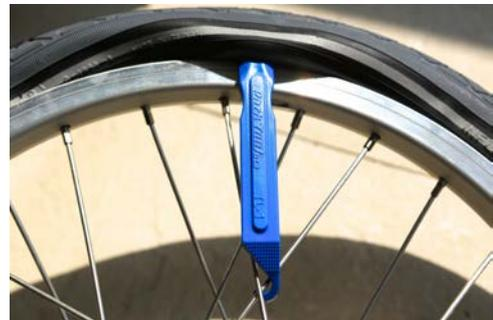
**Step 4.** Using another tire lever, scoop the bead wall next to the first lever and run along the rim to scoop out the entire bead wall of the tire.
