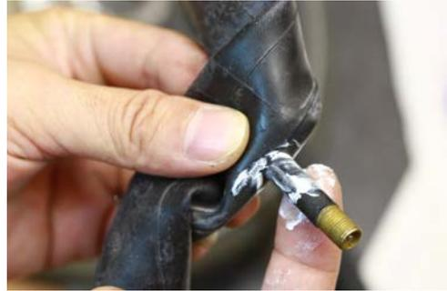
**Step 11.** Insert the valve stem of the inner tube through the rim tape first before going through the rim. You will have difficulty pushing in the valve stem through the rim without doing Step 10. Make sure the valve stem is completely inserted and is protruding straight and not slanted.
