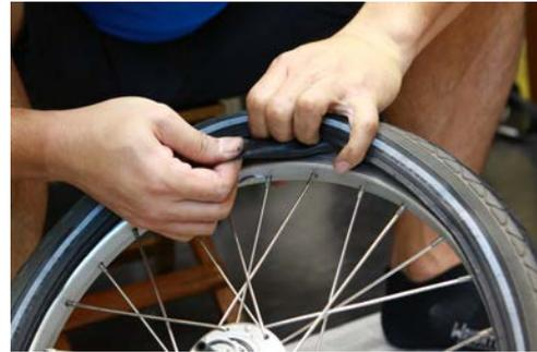
**Step 6.** Remove the tire from the rim completely.
