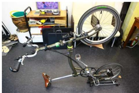
**Step 10.** Remove the 2 bolts and the 2 tab washers securing the rear wheel to the frame. Jiggle the rear wheel to loosen the tab washers if it is too tight for removal. Take note that the tab washers need to be re-installed in the correct orientation later. The “TOP” should be in the same orientation as the saddle side when bike is unfolded completely.
