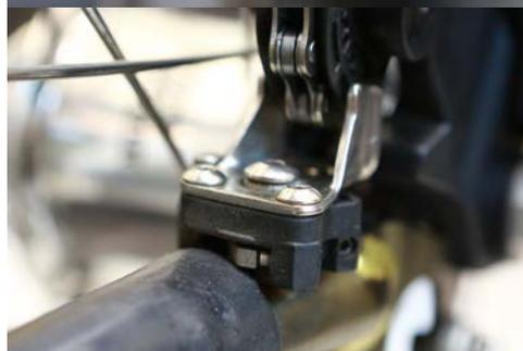
**Step 6.** Repeat Step 5 for the low gear lever position by adjusting the low limit screw. For the low limit screw, use the derailleur guide shown on the right as reference for adjustment.
