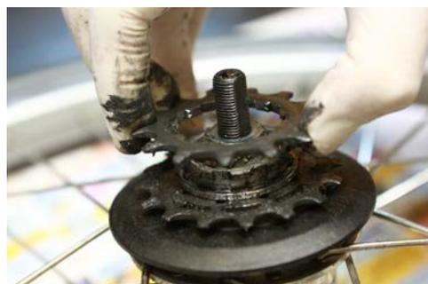
**Step 3.** Remove the spacer.
