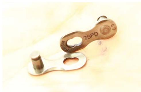
**Step 4.** To join the chain, install the links as shown.
