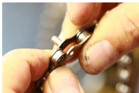
**Step 7.** Turn in the handle on the chain tool to position the push pin to just contact the chain pin on the chain. Make sure the push pin and the chain pin on the chain is aligned.
