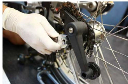
**Step 7.** Deflate the tire with the tip of the gear chain rod. This will allow the easy removal of the wheel from between the brakes.
