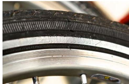
**Step 9.** Fit one side of the tire bead wall onto the rim as shown.
