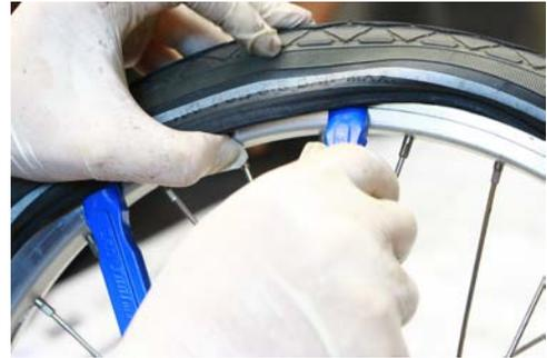
**Step 5.** Pull out the tube, starting from the opposite end of the valve stem and then remove the tube from the rim. Do not use excess force to pull out the tube as damage to the valve stem-tube interface is possible. You do not want to damage the tube especially if you need to fit on again later when changing to newer tires.
