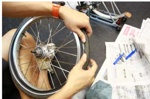
**Step 17.** You should be able to press fit the final section of the tire into the rim with a bit more effort after Step 16.
