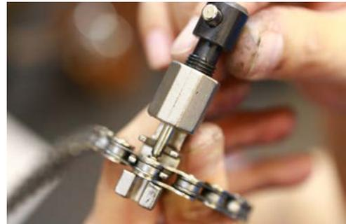
**Step 9.** Remove the chain from the lower chamber. You will notice that the chain link is very stiff and cannot be articulated. That is normal. Move the chain and the affected pin into the upper chamber as shown.
