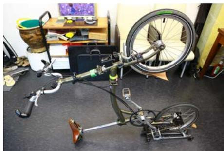
**Step 2.** Do a visual check on the gaps between the brake pads and the wheel rim. This should be done especially after a fall. The gaps should be roughly equal on both sides.
