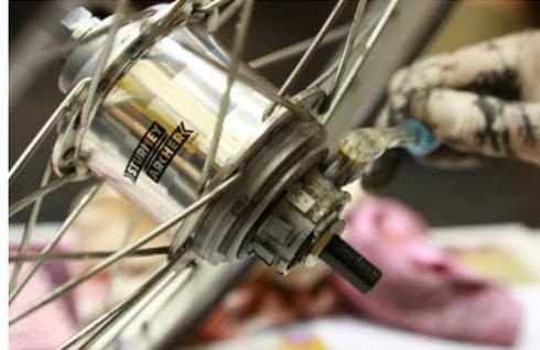
**Step 7.** To reinstall the components again, start by installing the plastic chain guard onto the hub. You should notice by now that the chain guard and sprockets are slotted to fit onto the hub only when correctly orientated with the splines. For quick orientation, look out for the smallest slot on the guard/sprockets and the corresponding spline on the hub.
