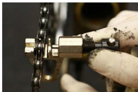
**Step 2.** Turn in the handle on the chain tool to position the push pin to just contact the pin on the chain. Make sure the push pin and the pin on the chain is aligned.
