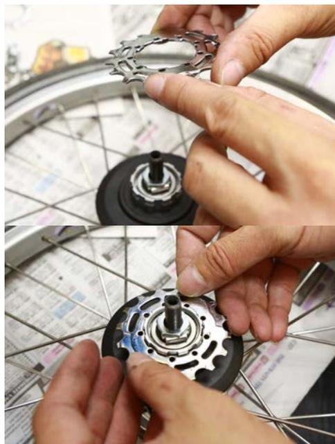
**Step 9.** Install the spacer.
