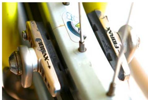
**Step 3.** In the unlikely event that it is out by a lot, centre the whole brake assembly. This can be done by loosening the bolt and re-tighten with a size 10mm spanner when done.
