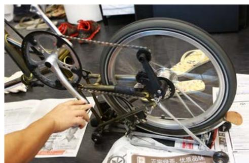
**Step 4.** Repeat step 3 with the next gear shift lever position. You should feel the change in resistance or sometimes hear a
