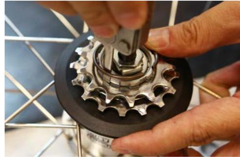
**Step 12.** Do a visual check to ensure the clip is installed properly. The re-installation process is now completed.
