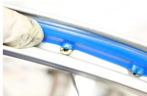
**Step 8.** To fit the tire back onto the rim, make sure you get the tire orientation correct because some tires are directional. For e.g., Schwalbe Marathon series. This is to avoid the effort to remove and install the tire again later.
