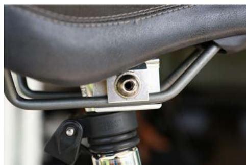
**Step 2.** Unfold the bike and lay the bike on one of its side to remove the seat post through the bottom of the seat tube.
