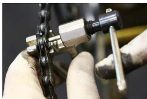
**Step 3.** Holding the chain and chain tool firmly, turn in the handle on the chain tool to push the chain pin out of the chain gradually. **DO NOT PUSH THE PIN OUT OF THE CHAIN COMPLETELY.** Else, the link will be unusable. The aim is to push out the chain pin just enough for the links on the chain to be separated.
