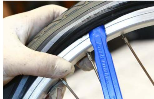
**Step 3.** Secure the hook end of the tire lever to one of the wheel spoke.
