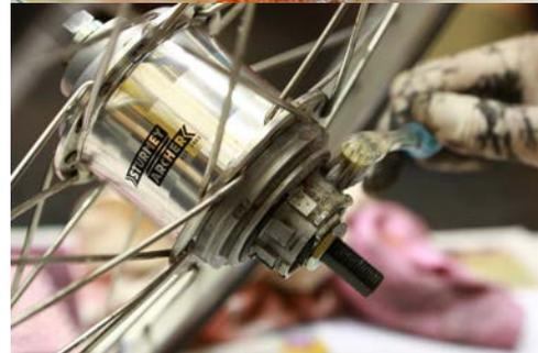
**Step 7.** To reinstall the components again, start by installing the plastic chain guard onto the hub. You should notice by now that the chain guard and sprockets are slotted to fit onto the hub only when correctly orientated with the splines. For quick orientation, look out for the smallest slot on the guard/sprockets and the corresponding spline on the hub.
