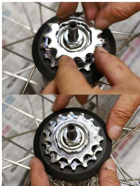
**Step 11.** To install the C-shaped spring clip to secure the sprocket assembly, hold down one side of the clip and use the flat head screwdriver to aid the installation process as shown.
