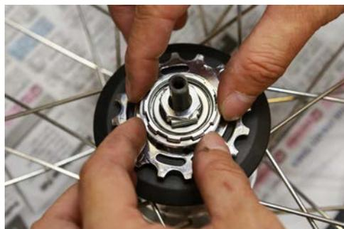
**Step 10.** Install the small sprocket with the correct orientation as shown.
